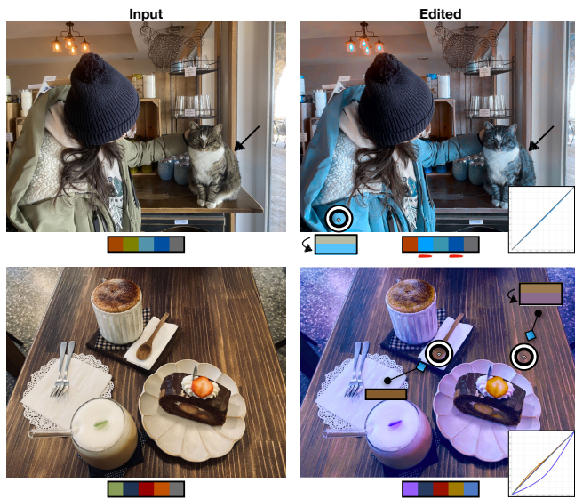
Fig. 12. Limitations of ColorfulCurves . First row: When different objects have similar colors, they may share a palette color. Changing the color on one object will apply similar color changes to the other objects (e.g. the woman’s jacket and cat). Second row: If two different image-space constraints are placed on pixels with similar input colors, ColorfulCurves is unable to find a palette satisfying both constraints simultaneously without drastic, undesirable changes elsewhere (e.g. the spoon and table).
