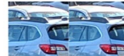
Fig. 7. Anisotropic Kernels. Left: When isotropic kernels ( k_{x,iso} = 1 , k_{y,iso} = 1 ), only a global mean will be used, small weight differences cause blurry edges along edges. Right: Anisotropic kernels ( k_{x,iso} = 0 , k_{y,iso} = 1 ) in the center.
