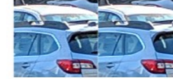
Fig. 7. Anisotropic Kernels. Left: When isotropic kernels ( \beta_{\text{horizontal}} = 1 , \beta_{\text{vertical}} = 1 ) are applied to an image, small misalignments cause blurry edges. Right: Anisotropic kernels ( \beta_{\text{horizontal}} = 0 , \beta_{\text{vertical}} = 1 ) in the corners.
