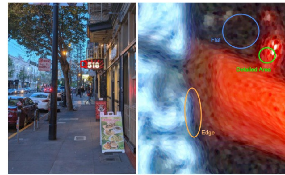
Fig. 6. Sparse data reconstruction with anisotropic kernels: Exaggerated example of very sharp (i.e., narrow, k_{detail} = 0.05px ) kernels on a real captured burst. For demonstration purposes, we represent samples corresponding to whole RGB input pictures instead of separate color channels. Kernel adaptation allows us to apply differently shaped kernels on edges (orange), flat (blue) or detailed areas (green). The orange kernel is aligned with the edge, the blue one covers a large area as the region is flat, and the green one is small to enhance the resolution in the presence of details.
