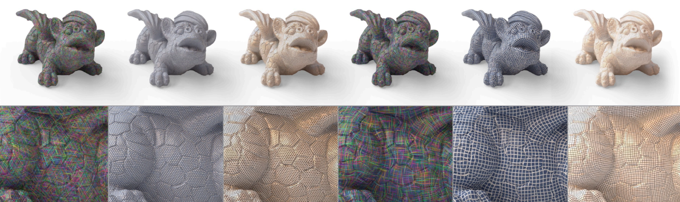
Figure 1: Remeshing a scanned dragon with 13 million vertices into feature-aligned isotropic triangle and quad meshes with ~80k vertices. From left to right, for both cases: visualizations of the orientation field, position field, and the output mesh (computed in 71.1 and 67.2 seconds, respectively). For the quad case, we optimize for a quad-dominant mesh at quarter resolution and subdivide once to obtain a pure quad mesh.
