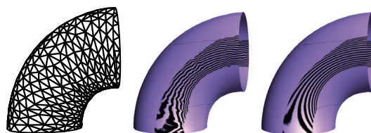
Figure 1: A mesh (left) optimized using cotangent formula mean curvature discretization (middle) and using midedge normal-based curvature functional (right).
