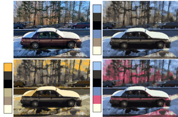
Figure 3: We create posterized images (top right) using blended colors from an automatically chosen palette, computing per-pixel additive mixing weights for the palette. Users can edit the palette (bottom row), to re-color the posterized image by re-mixing the per-pixel weighted palette in real-time.
